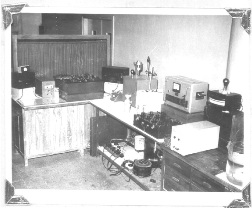
Experimental set up for D.C. resistivity measurements
