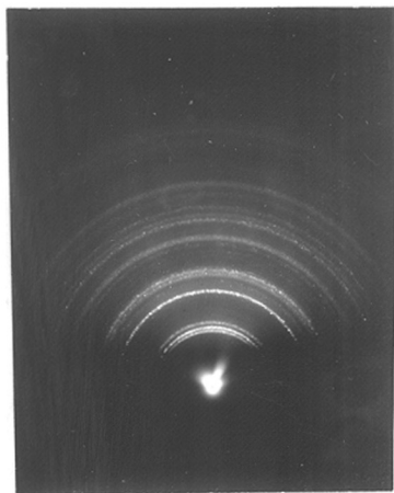
Fig. 24. macrocrystalline cupric sulphide resulting from action of sulphur upon alpha brass at 250°C.
