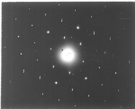
Fig. 27. "Reflection" pattern from projecting flake upon a copper surface exposed to sulphur at 160°C. The pattern results from transmission through the basal planes of hexagonal cupric sulphide.
