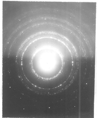
Fig. 26. Macrocrystalline cupric sulphide from action of sulphur upon brass at 300°C. (Reflection pattern, but projecting flakes at lower edge throw a pattern behind the shadow edge.
