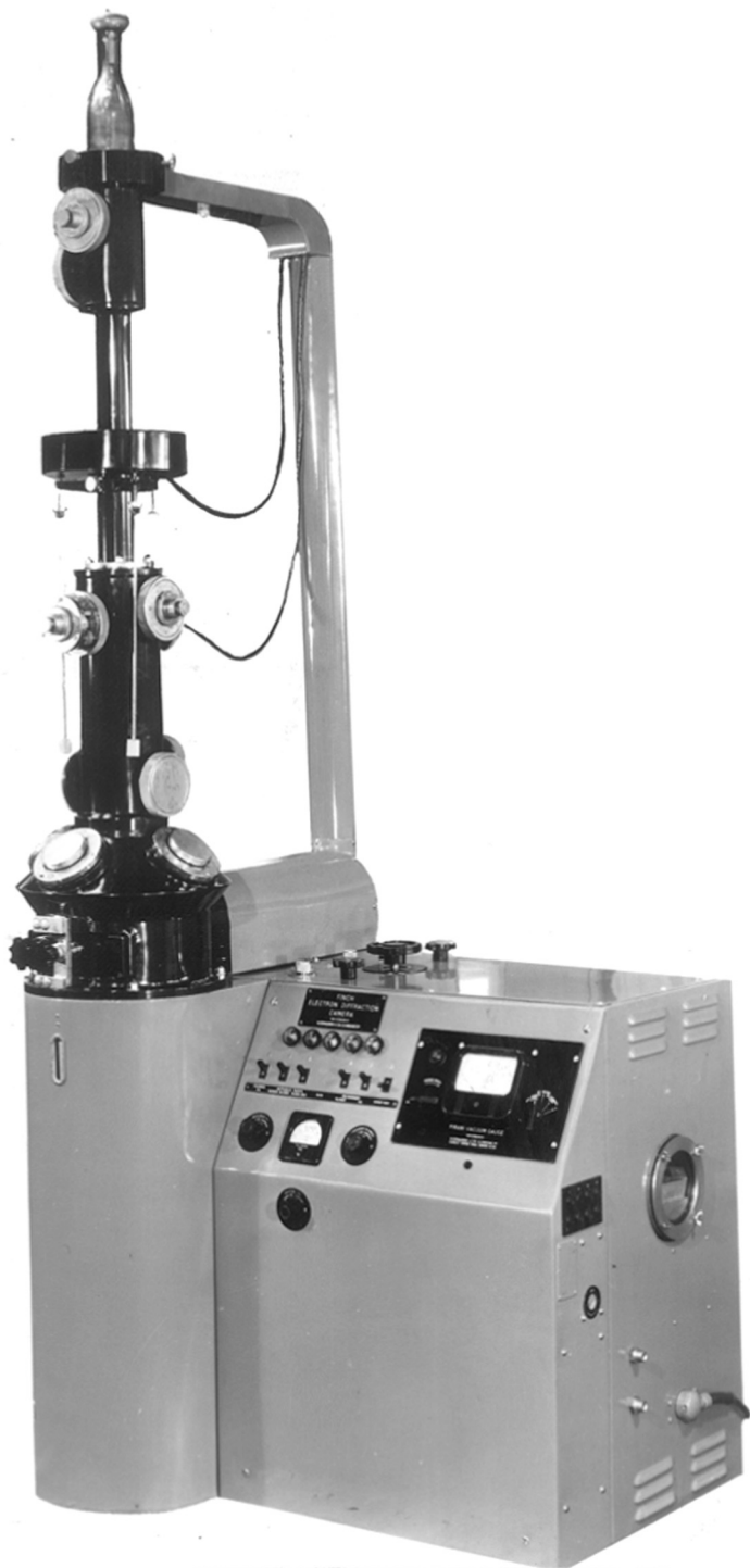
Fig.(5) Finch Electronic Diffraction Camera - Commercial Pattern (W.Edwards & Co. - London ).
