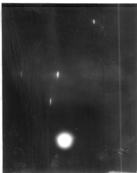
Fig.(42) Macrocrystalline electropolished aluminium (a and b represent different parts of the specimen.
