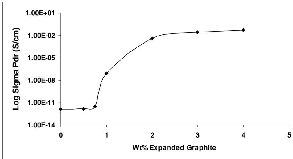
**Figure 5.3.5.** DC conductivity of PP-7 wt% graphite-ExGr composites
