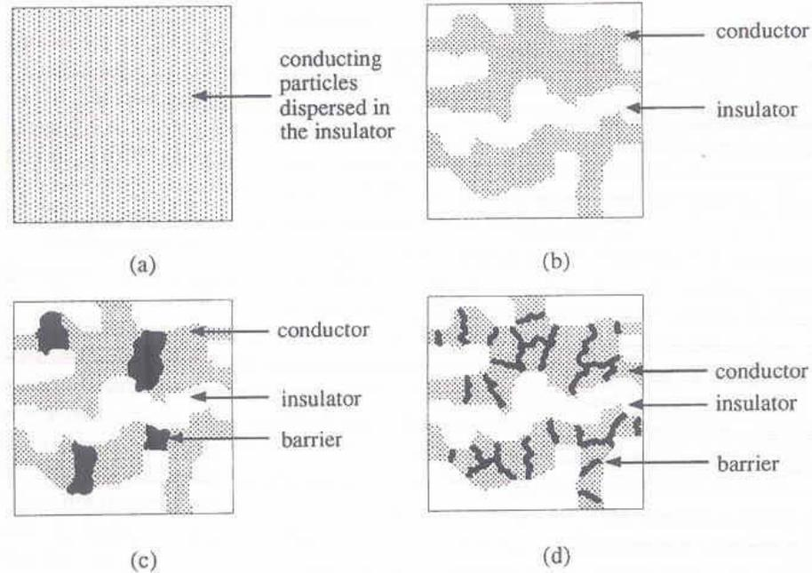
**Figure.1.6.** a) Uniform model b) Uniform channel model c) Non-tunneling barrier model d) Tunneling barrier model
