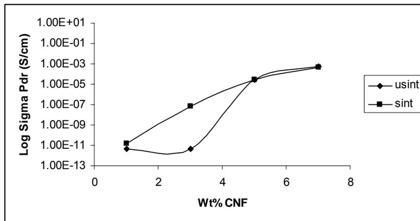
**Figure 3.2.4.** Through plane conductivity of PES-CNF composites before and after sintering
