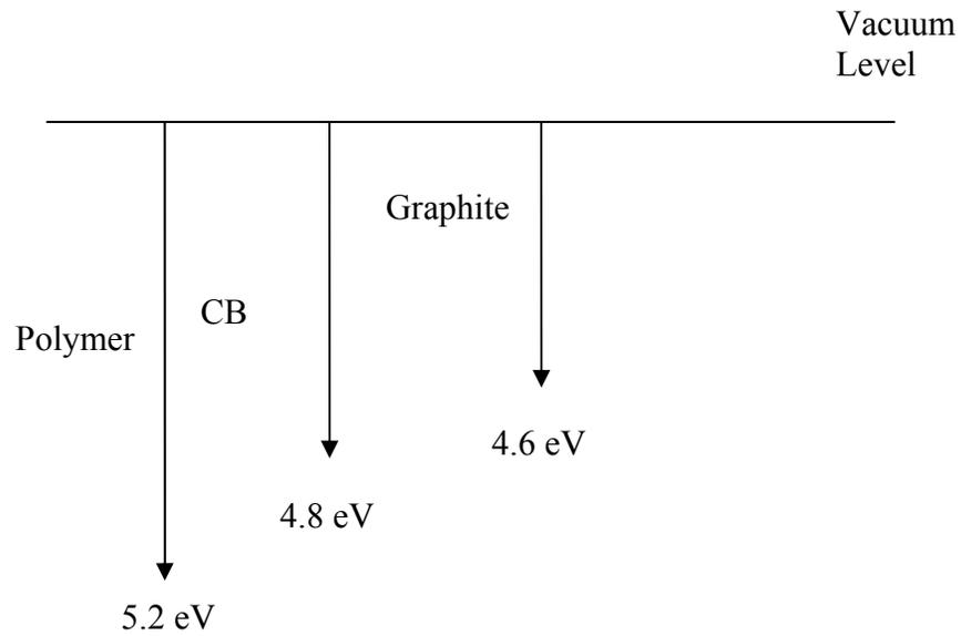
**Figure 4.2.13.** Work function diagram of fillers
