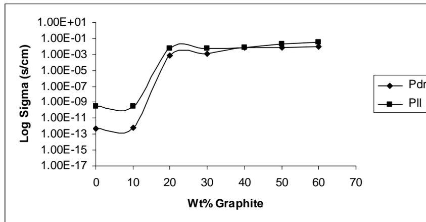
**Figure 4.5.** DC conductivity of melt crystallized PPS-graphite composites
