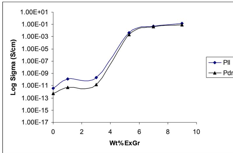
**Figure 3.3.3.** DC conductivity of PES-expanded graphite composites
