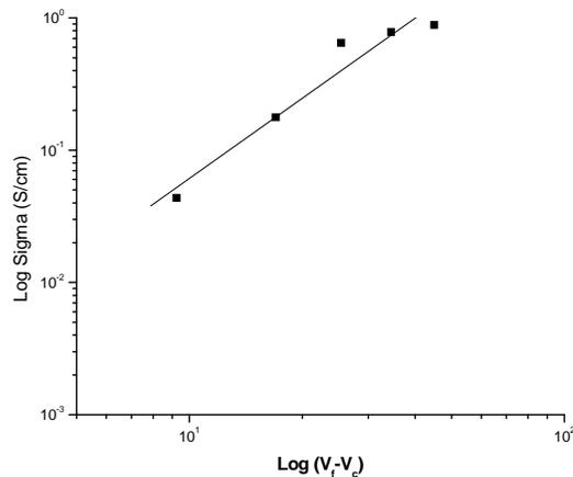
**Figure 4.2.2.** Plot for determination of percolation exponent in PPS-graphite composites
