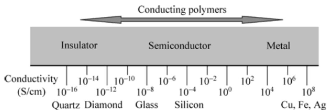
**Figure 1.3.** The range of conductivities of conducting polymers including doping
