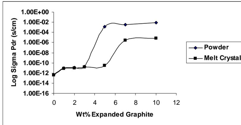
**Figure 4.5.1.** Effect of preparation routes on the through plane conductivity of melt crystallized PPS-ExGr composites
