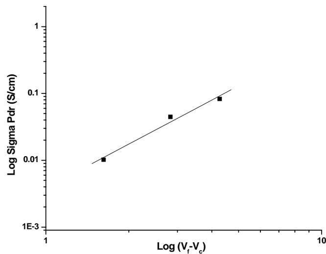
**Figure 3.3.4.** Plot for extracting percolation exponent of PES-expanded graphite composites
