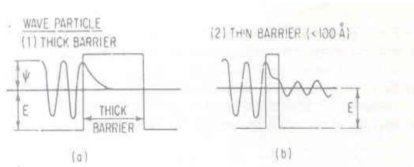
**Figure. 1.8.** Tunneling conduction a) thick barrier b) thin barrier
