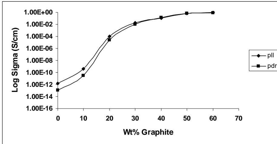
**Figure 5.2.1.** DC conductivity of PP-graphite composites
