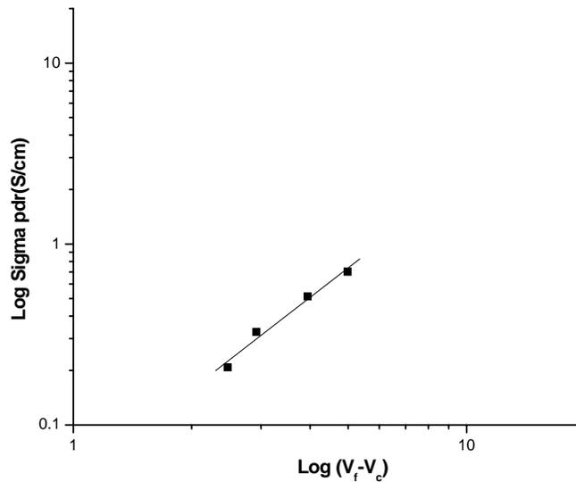
**Figure 5.3.2.** Log  $\sigma_{pdr}$  vs Log ( $V_f - V_c$ ) plot of PP-ExGr composites
