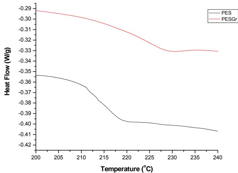
**Figure 3.1.19.** DSC curves of PES and PES-38 wt% graphite solution blended samples
