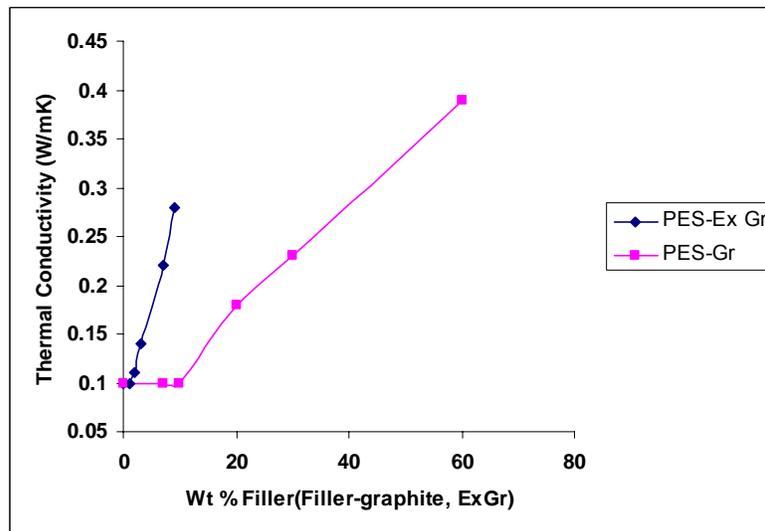
**Figure 3.5.2.** Thermal conductivity of PES-ExGr and PES-graphite composites
