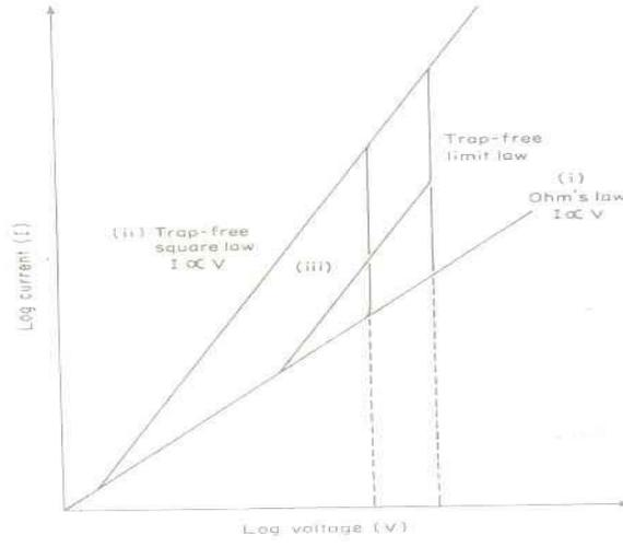
**Figure. 1.10.** I-V Characteristics of a solid with space charge conduction
