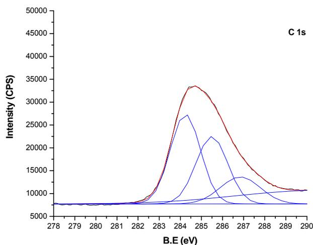
**Figure 3.1.16.** C 1s core level spectrum of graphite in PES
