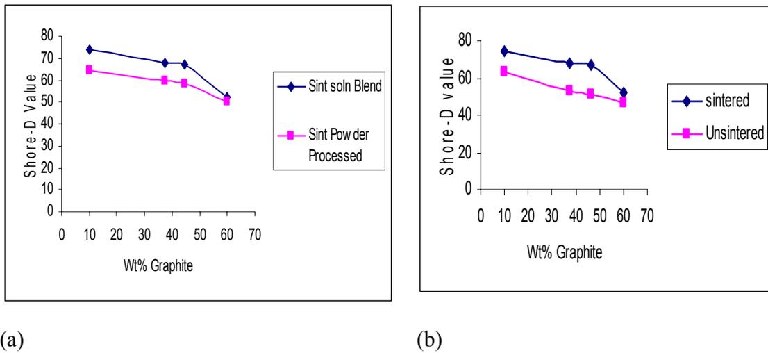
**Figure 3.1.11.** Hardness of PES-graphite composites a) Effect of processing routes b) Effect of sintering
