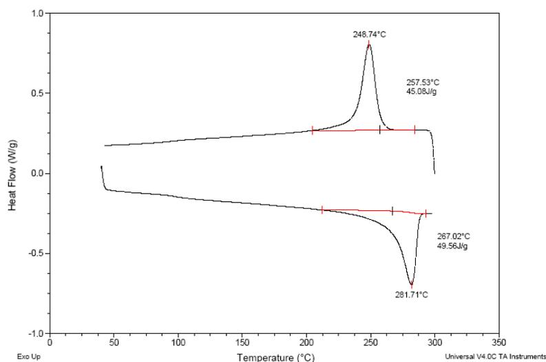
**Figure 4.4.6.** DSC of PPS-0.5 wt% CNF
