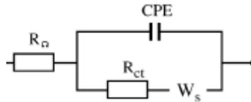
**Figure. 1.14.** Equivalent circuit diagram for ORR in fuel cell
