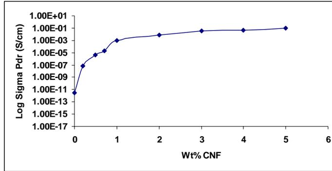
**Figure 5.4.4.** Through plane conductivity of PP-7 wt% graphite-CNF composites. After 1 wt% CNF in PP-7 wt% graphite, saturation in the conductivity is obtained due to completion in the network formation.
