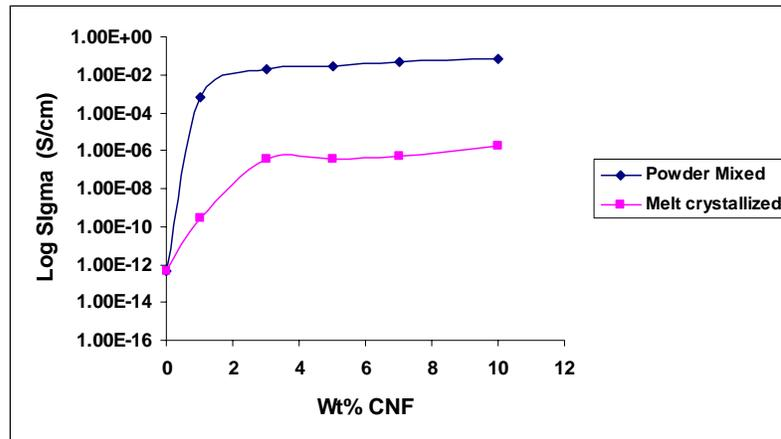
**Figure 4.5.4.** Effect of preparation route on the through plane conductivity of PPS-CNF composites
