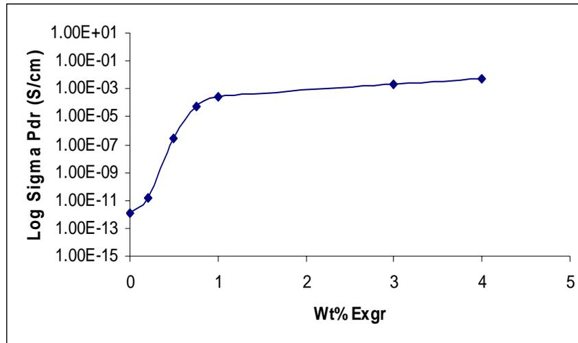
**Figure 4.3.8.** DC conductivity of PPS-graphite-ExGr hybrid composites
