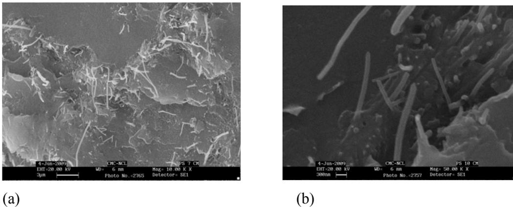
**Figure 4.5.6.** SEM pictures of melt crystallized a) PPS-7 wt% CNF b) PPS-10 wt% CNF composites
