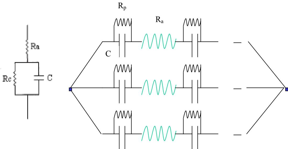
**Figure 3.1.24.** Model of conducting polymer composites
