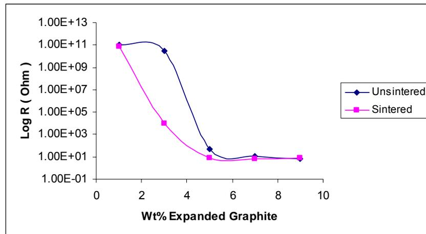
**Figure 3.3.5.** Through plane resistance of PES-ExGr composites (Sample thickness 5 mm, area 1cm<sup>2</sup>)
