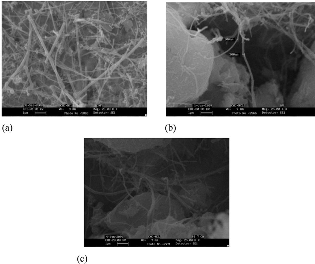
**Figure 4.4.4.** SEM pictures of a) Pure CNF b) Unsintered c) Sintered PPS-3 wt% CNF composites
