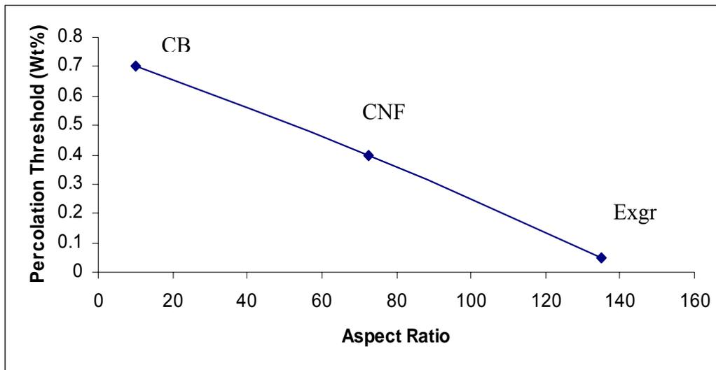
**Figure 3.4.1.** Effect of aspect ratio of second filler in PES-graphite based composites
