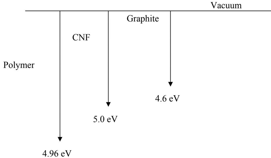
**Figure 3.2.12.** Work function diagram
