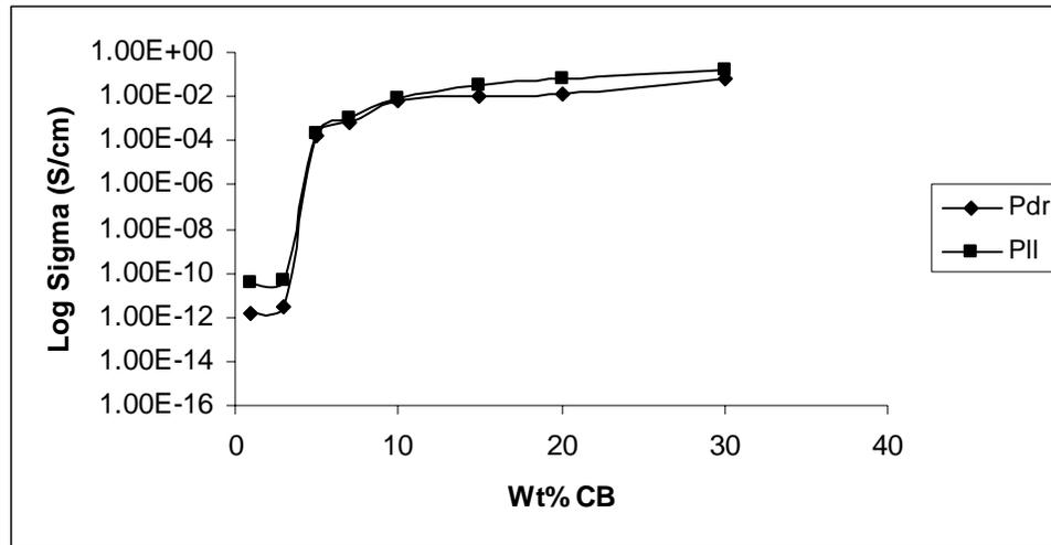
**Figure 4.2.9.** DC conductivity of powder mixed PPS-CB composites
