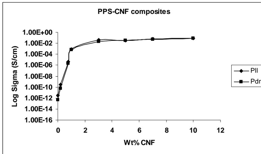
**Figure 4.4.1.** DC conductivity of powder mixed PPS-CNF composites
