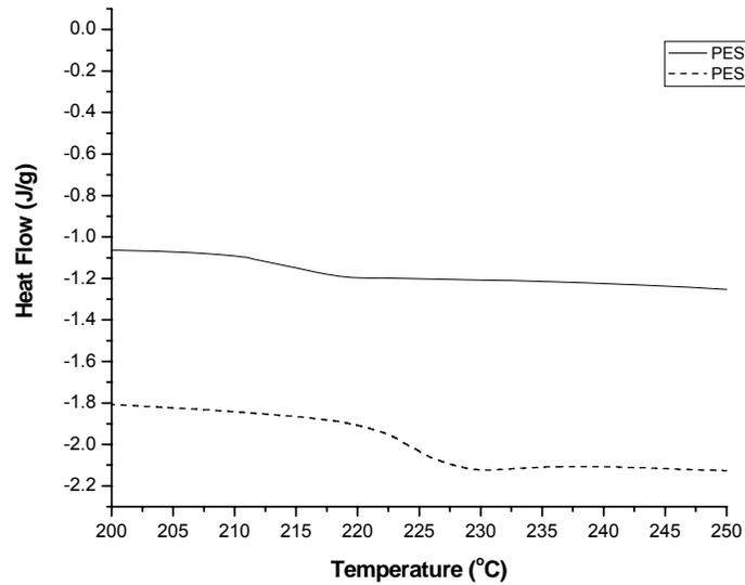
**Figure 3.2.7.** DSC comparison between pure PES and PES-5 wt% CNF
