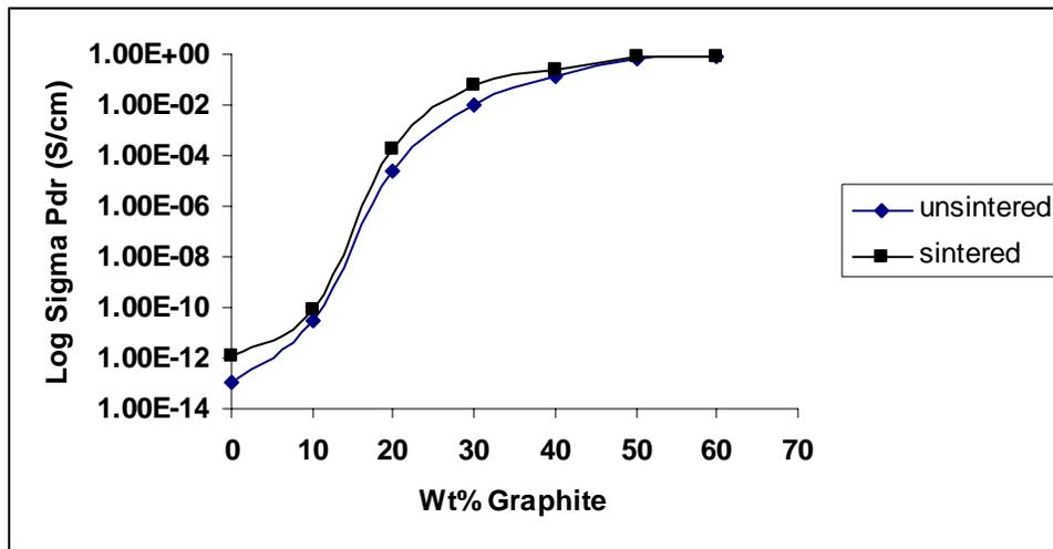
Figure 5.2.3. Through plane conductivity of PP-graphite composites before and after sintering
