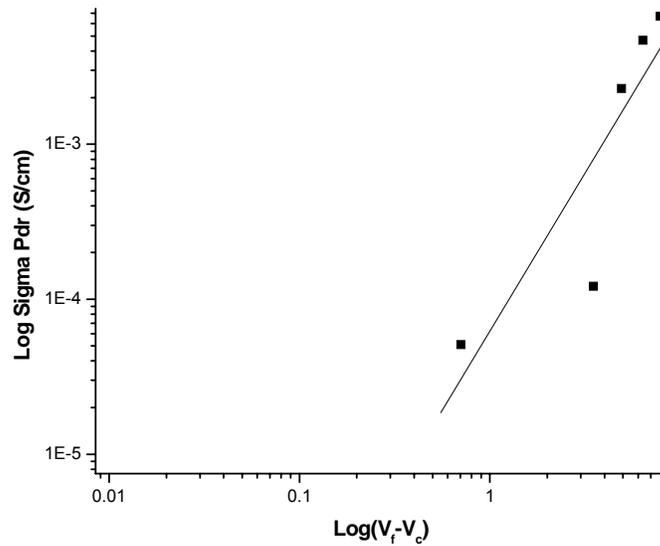
**Figure 3.2.3.** Log-Log plot of through plane conductivity vs volume fraction of CNF in PES
