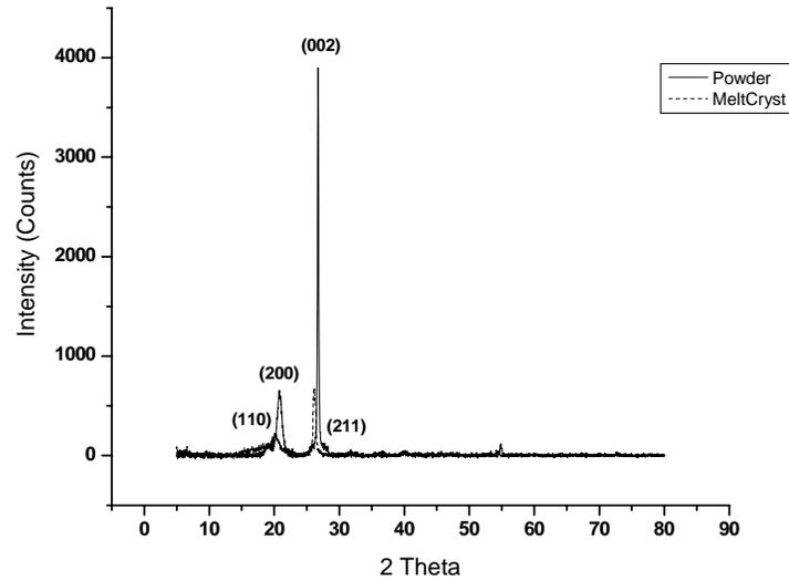
**Figure 4.5.3.** XRD of PPS-7 wt% graphite melt crystallized sample
