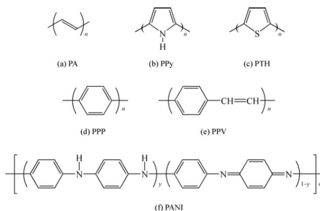
**Figure. 1.2.** Molecular structure of typical conducting polymers
