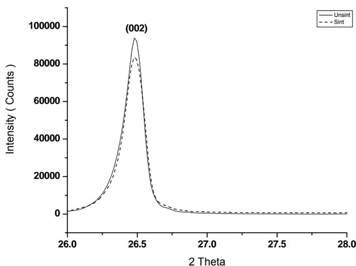
**Figure 3.1.13.** XRD pattern of graphite part of PMMA-Graphite composites
