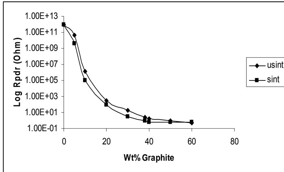
**Figure 3.1.10.** Through plane resistance of PES-graphite solution blended composites before and after sintering
