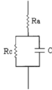
**Figure. 1.12.** Equivalent circuit of CPCs
