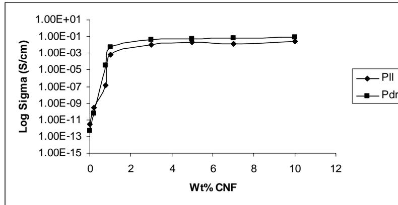
**Figure 4.4.2.** DC conductivity of PPS-CNF composites after sintering
