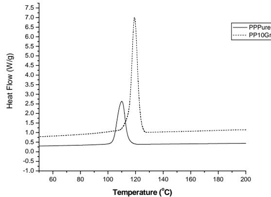
**Figure 5.2.11.** DSC cooling curve of PP and PP-10 wt% graphite
