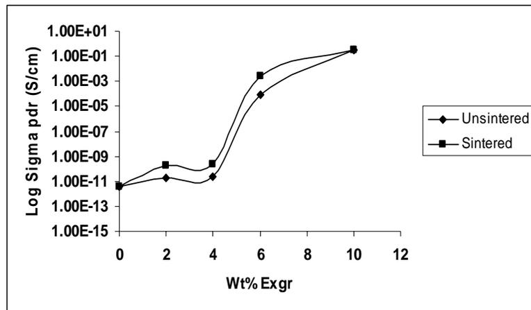
**Figure 5.3.3.** Through plane conductivity variation before and after sintering of PP-ExGr composites
