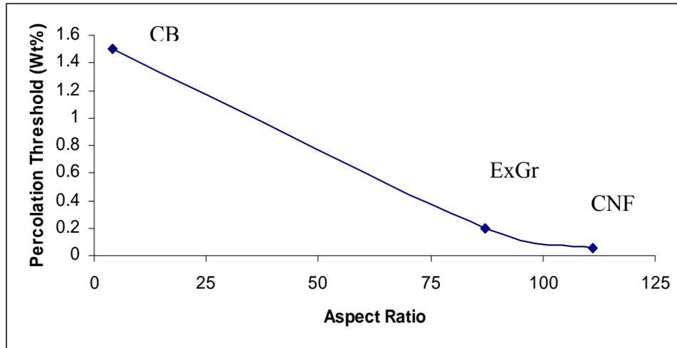
**Figure 4.4.10.** Effect of aspect ratio of second conducting fillers on electrical percolation threshold
