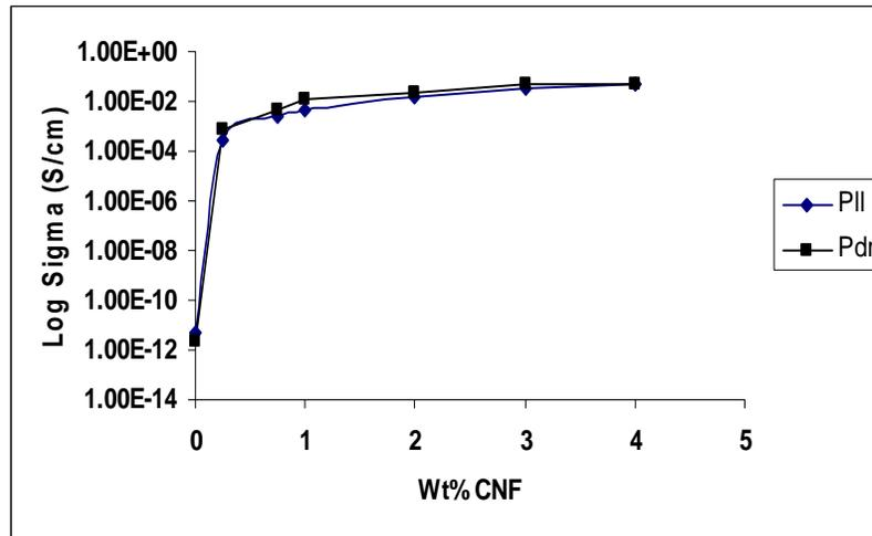
Figure 4.4.7. DC conductivity of PPS-7 wt% graphite- CNF composites
