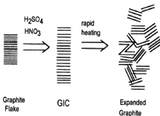
**Figure 3.3.2.** Expanded graphite synthesis
