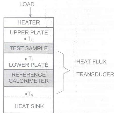
**Figure. 2.2.** Thermal conductivity test meter schematic
