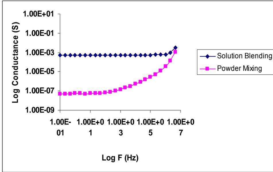
**Figure 3.1.21.** Effect of preparation route on electrical conductance of PES-7wt% graphite-2 wt% CB
