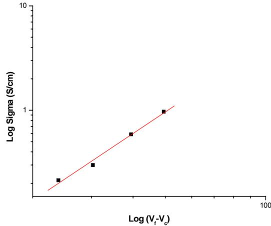
**Figure 3.1.12.** Log-Log plot of through plane conductivity vs volume fraction of graphite in PES
