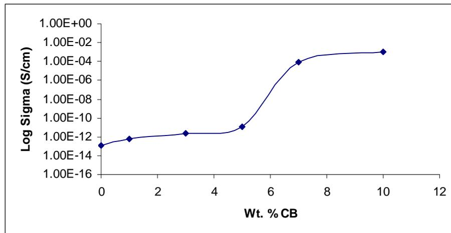
**Figure 5.2.7.** DC conductivity variation of PP-CB powder mixed composites
