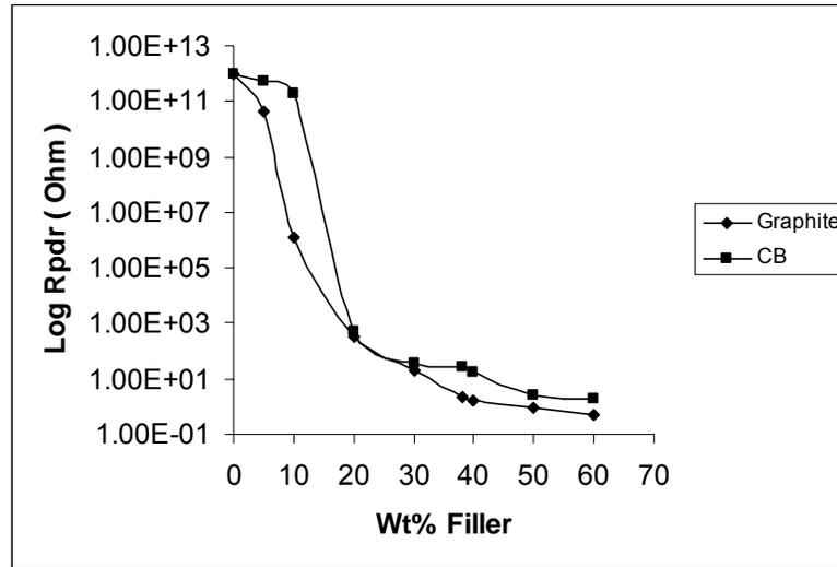
**Figure 3.1.2.** Through plane resistance variation of PES-Graphite, PES-CB solution blended composites
