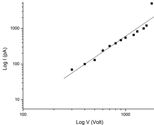
**Figure 3.1.28.** I-V Characteristics of PES-graphite-PES single junction
