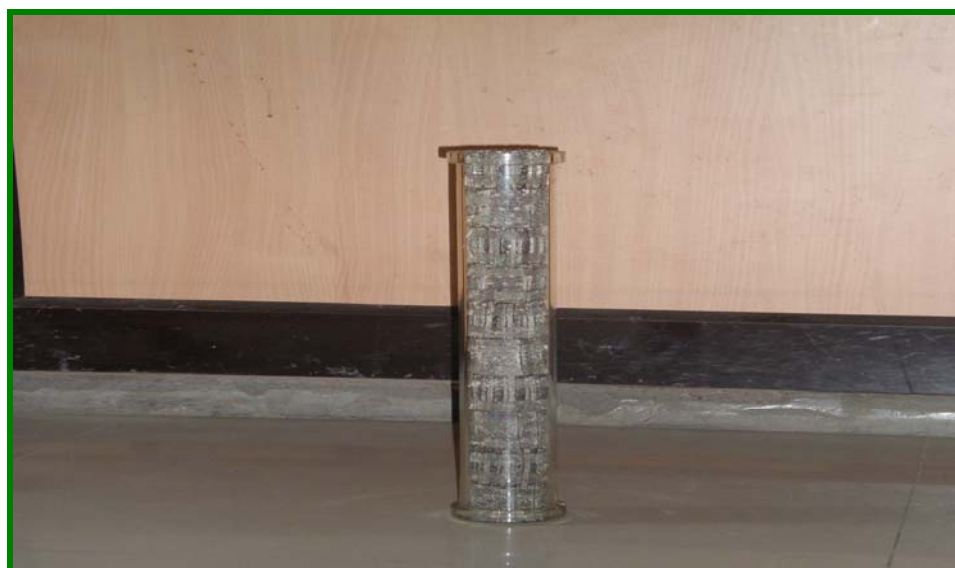
Figure 5.6 Catalyst Packed Columns for Reactive Section
