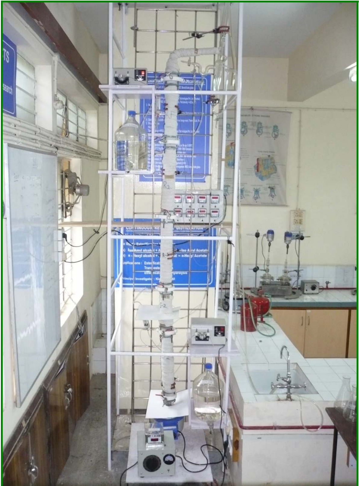
Figure 5.2 Photograph of Experimental Setup for Continuous Reactive Distillation Column, which is functional at Petrochemical Processes Lab. at MIT, Pune, India
