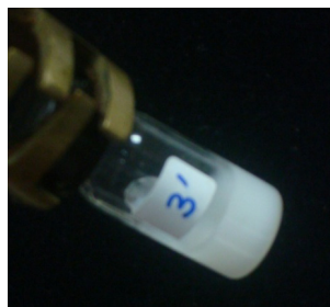
Figure 5.5. Snapshot of sample of 5% PEI in 47.5%/47.5% (by weight) C_{12}E_9/H_2O at 25°C at pH 1.
