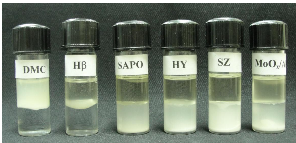
Fig. 3.8. Preferential dispersion of DMC in non-polar, soybean oil layer, H \beta near the interface and HY, SAPO-11, sulfated zirconia (SZ) and MoO x /Al 2 O 3 in polar water layer
