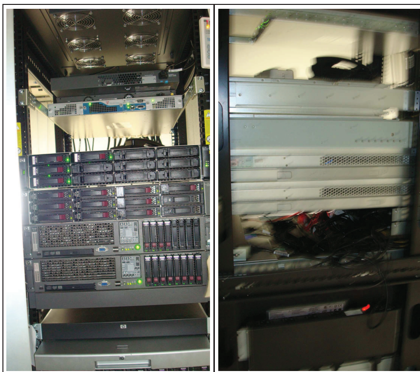
FIGURE 2.1: The 128 cores Intel(R) Xeon(R) CPU 5160@3.00GHz cluster computer - BOSE, used mainly for the work in this thesis.
