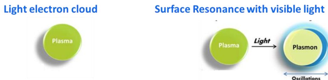
Figure 1.4: Surface plasmon resonance in the presence of visible light.
