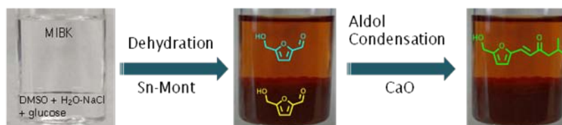
Figure 4.2.6. Formations of aldol product in MIBK phase enabling clean/easy product separation and isolation.
