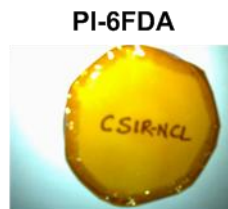
Figure 4a.2 PI-6FDA film cast from chloroform
