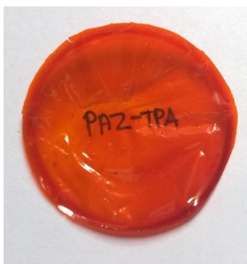
Figure 4c.2 PAZ-TPA film cast from chloroform
