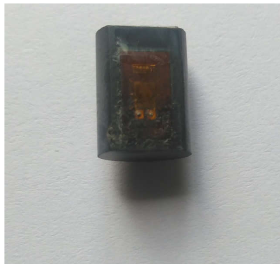
Figure 2.4: Photograph of a sintered cylindrical shaped pellet with strain gauge cemented on it, used for the magnetostriction measurements.
