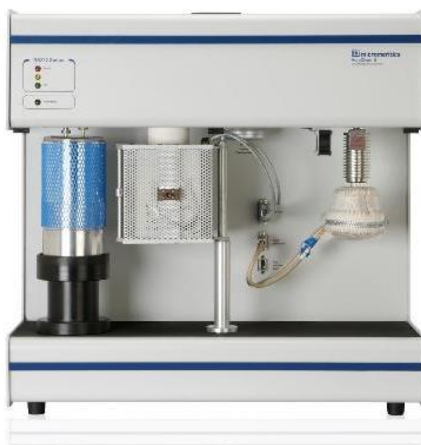
Fig. 2.4. Micromeritics Autochem 2920 instrument used for TPR/TPO.
