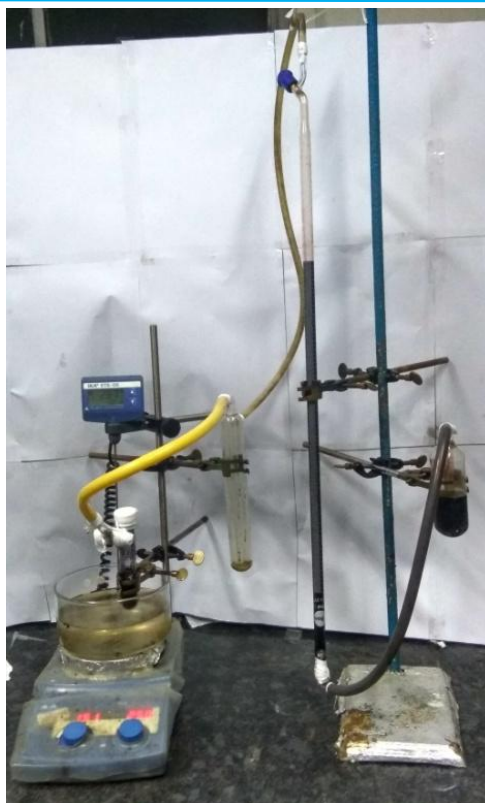
Figure 2A.17. Setup for hydrogen gas evolution (a volumetric quantitative analysis).
