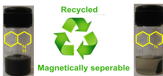
Figure 2A.19. Digital photograph showing a) the fine dispersion, and b) magnetic separation of Fe-L1@EGO-900.
