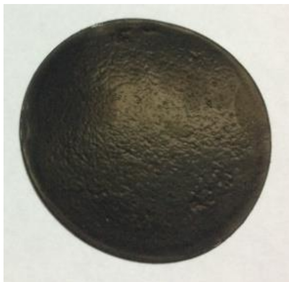
Figure 1. Photograph of the free-standing electrode made from the CNT-PEDOT composite.
