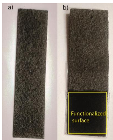
Figure 1. Digital photographs of a) pristine Toray carbon paper (pT); b) functionalized Toray carbon paper (fT). After functionalization, the surface of the Toray paper turns dark which can be seen in the above images.
