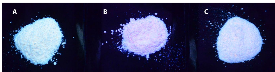
Figure 4A.10: Optical images showing emission from (A) PS-NH 2 and (B) PS-KPS (C) PS-COOH observed under UV lamp.
