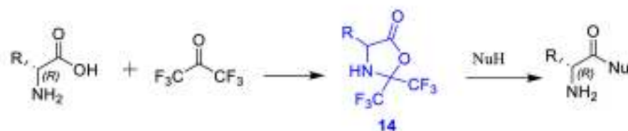
Scheme 2: One step amidation reaction of amino acid with hexafluoroacetone as simultaneous protecting and activating agent.
