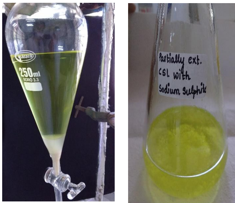
Fig 5: (a) Separation of cell mass from the solvent phase (b) Partially extracted CSL with sodium sulphate crystals.
