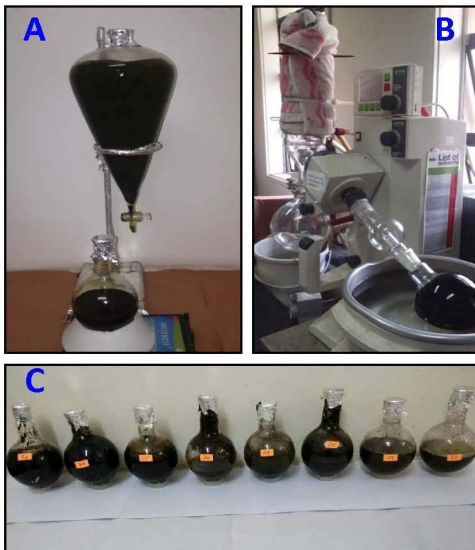
Fig.2.2-A: Plant extraction, B: Evaporation and C: Plant extracts stored in RB flasks
