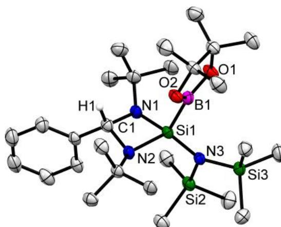
**Figure 1.** Molecular structure of **8**. Anisotropic displacement parameters are depicted at the 50% probability level. Hydrogen atoms (except H1 bonded to C1) are omitted for clarity. Selected bond distances (Å) and bond angles (deg): C1–H1 1.00(5), Si1–B1 2.031(5), Si1–N1 1.743(3), Si1–N2 1.742(3), Si1–N3 1.740(4); N1–Si1–B1 109.8(2), N2–Si1–B1 114.4(2), N3–Si1–B1 113.2(2), N1–Si1–N2 77.4(2), N1–Si1–N3 120.1(2).
