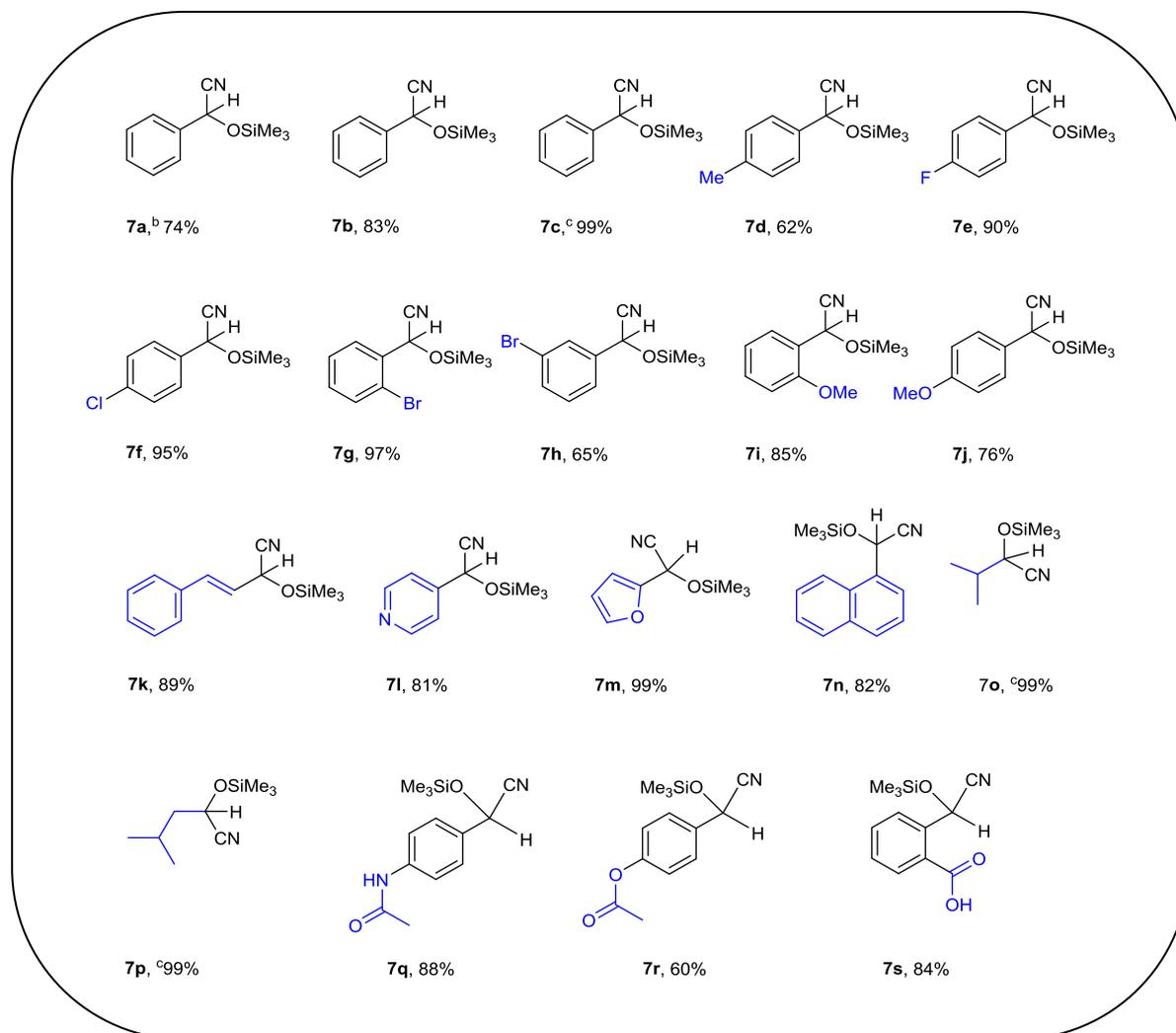
**Scheme 3.** <sup>a</sup>Reaction conditions: 3 mol% catalyst, 6h reaction at room temperature in benzene. Yields were determined by NMR spectroscopy on the basis of the consumption of the aldehyde. <sup>b</sup>2 mol% catalyst; <sup>c</sup>heating at 55 °C.
