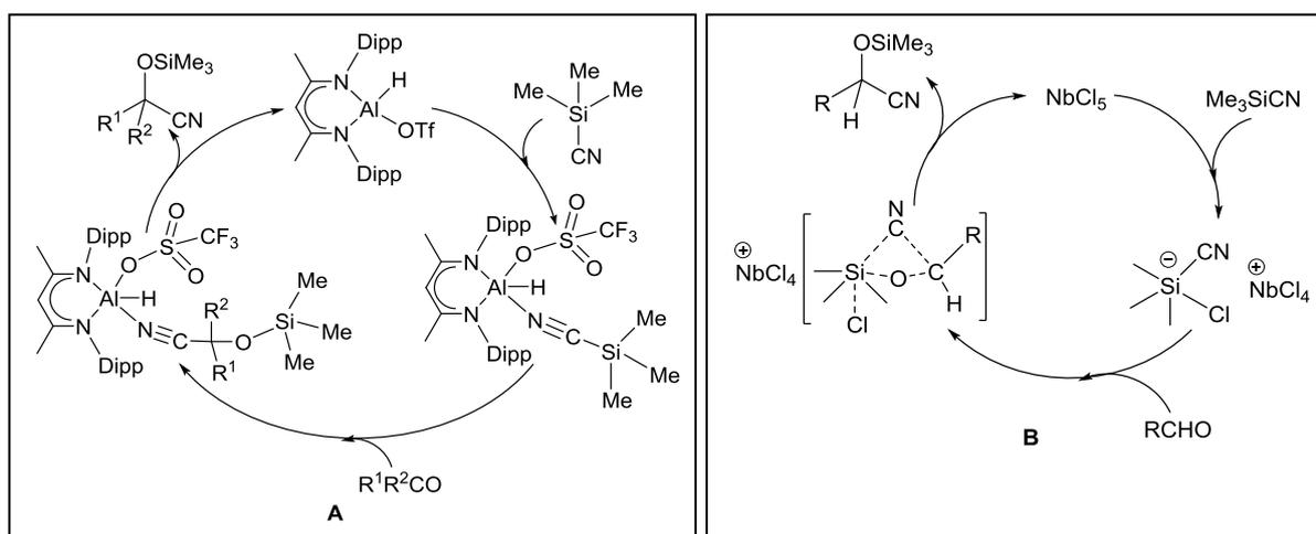
**Scheme 4.** Mechanism **A** was proposed by Zhi, Parameswaran, and Roesky and their co-workers for the operation of the  $\text{NaCNacAlH}(\text{OTf})$  catalyst. Mechanism **B** was proposed by George and Kim for cyanosilylation of carbonyl compounds catalyzed by  $\text{NbCl}_5$ .
