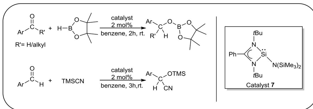
**Scheme 1.** S(II) catalyzed hydroboration of carbonyl compounds and cyanosilylation of aldehydes.
