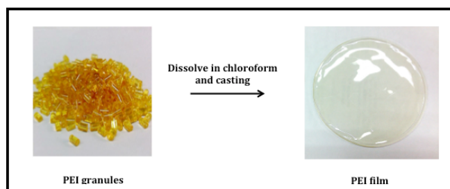
Figure. 2.1: Conversion of PEI beads to a film.
