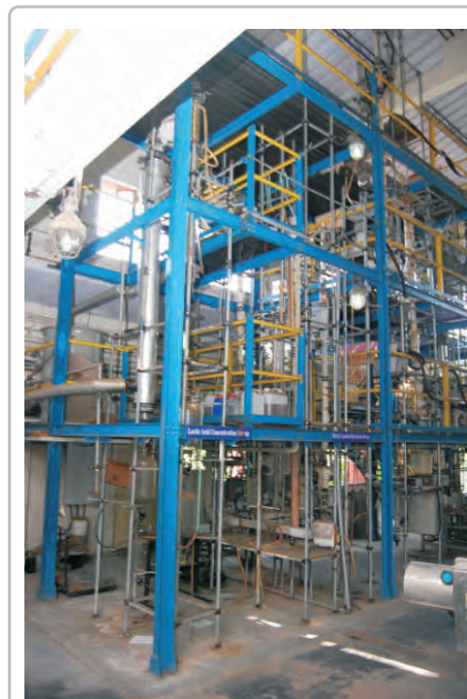
Continuous production of lactic acid process at pilot plant scale in NCL
