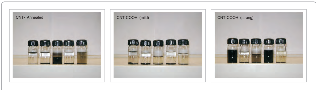
Photographs of carbon nanotube dispersion in various solvents – visual examination (1 - Water, 2 - Toluene, 3 - THF, 4 - Methanol, 5 - Acetone)
