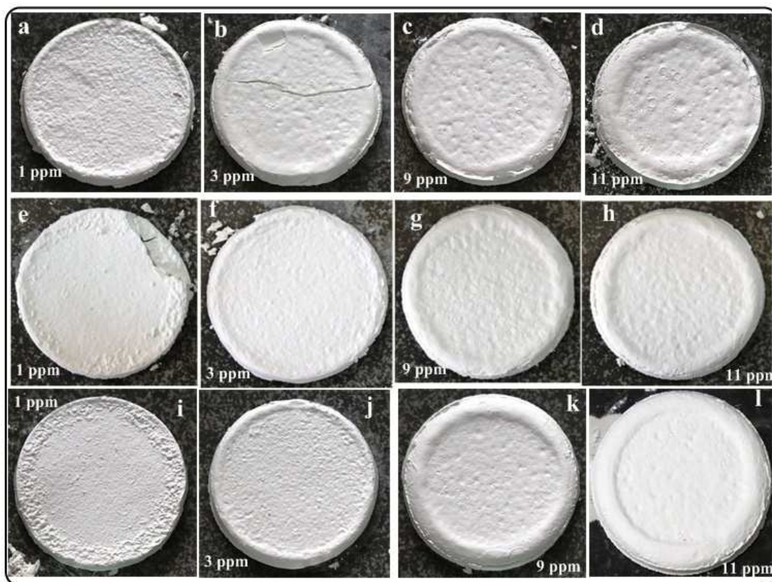
Figure-4.13: Photographs of filter cakes after flocculation and drying for AA-4060 (a-d) AA-5050 (e - h) and AA-8020 (i-l)
