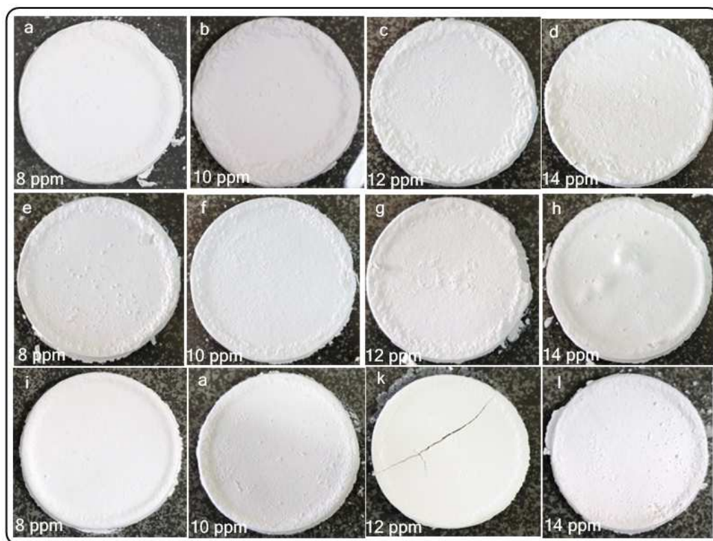
Figure-3.16: Photographs of filter cakes after flocculation and drying for AD-8020 (a-d) AD-5050 (e - h) and AD-4060 (i-l)
