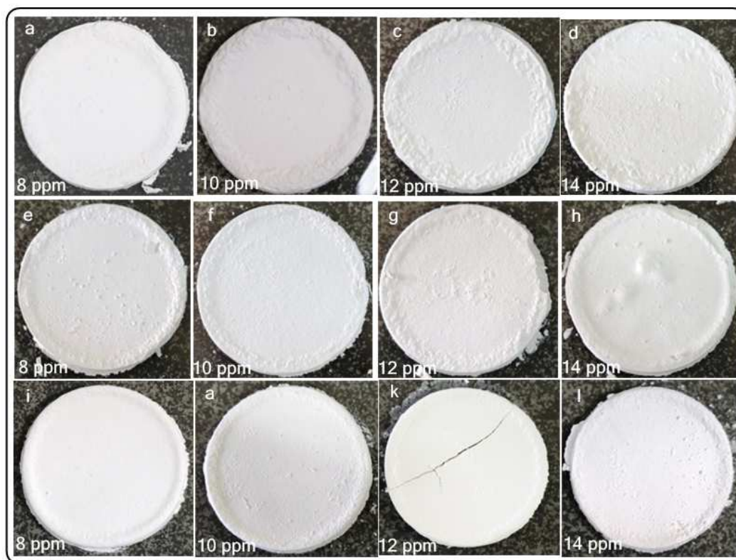
Figure-3.16: Photographs of filter cakes after flocculation and drying for AD-8020 (a-d) AD-5050 (e - h) and AD-4060 (i-l)
