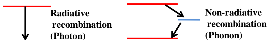
Figure 2.10: shows possible luminescence pathways in semiconductor
