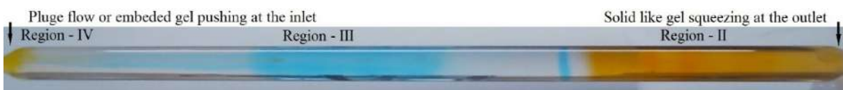
Figure A.5 Time dependent (i) pressure evolution and (ii) - (ix) simultaneous flow visualization with a dye inside the pipe ( D = 1\text{cm} , l = 30\text{cm} ) during suspension flow ( C_{lap} = 2.4\text{wt}\% & C_s =
