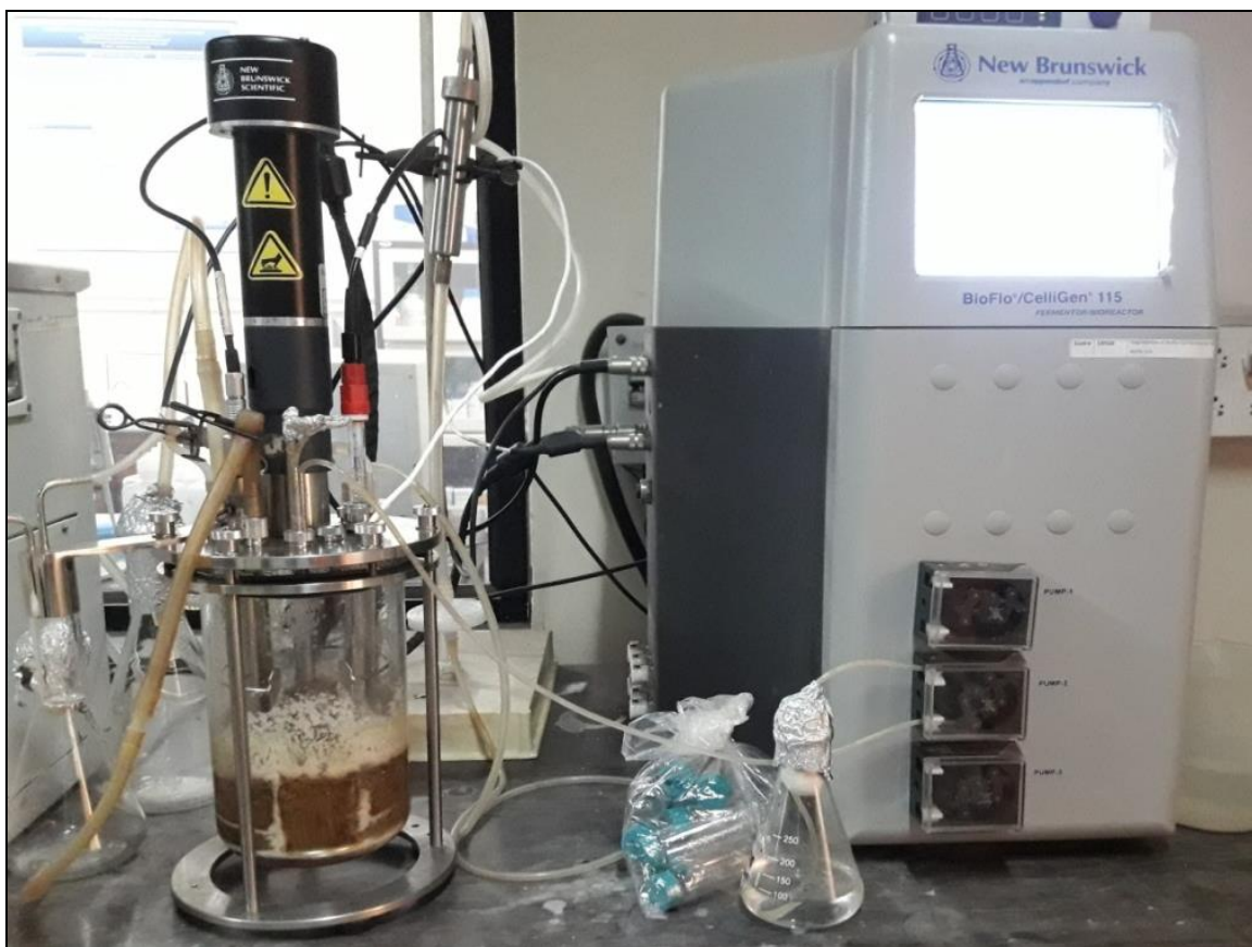
Figure 3.3 Batch Fermentation for B. poitrasii biomass production (New Brunswick BioFlo®/CelliGen® 115, Germany) (Fermenter was programmed at agitation from 250-400 rpm, aeration 2.5 lpm, initial pH 6.5, temperature, 28 °C for 48 h).
