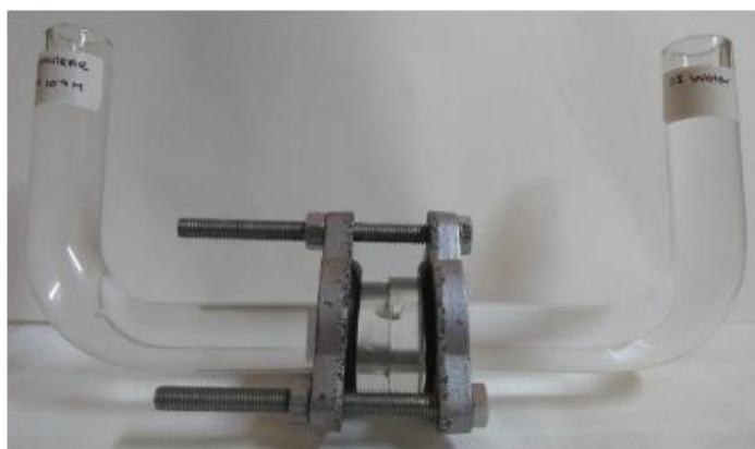
Figure 2.1 Naphthalene transport study through membranes using U-tube setup
