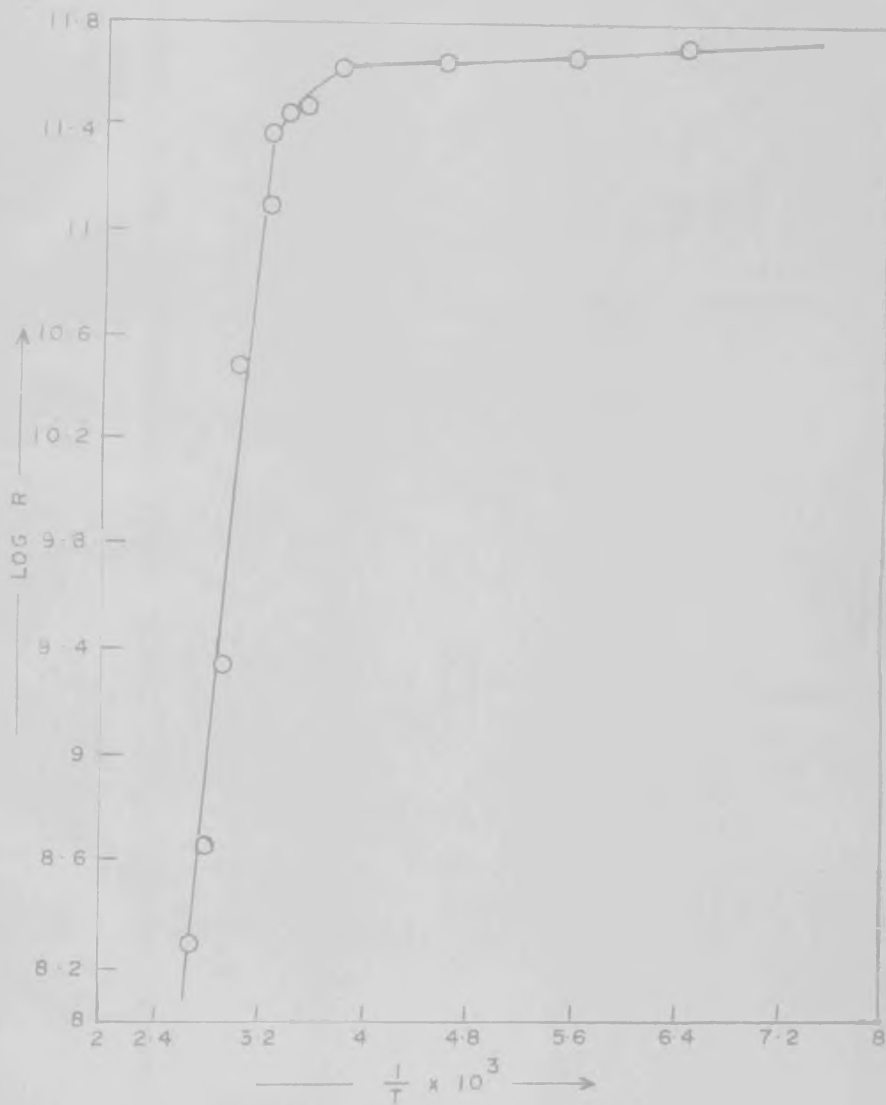
Fig 2.5 LOG DARK RESISTANCE VS \frac{1}{T} PLOT FOR CdS THIN FILM
