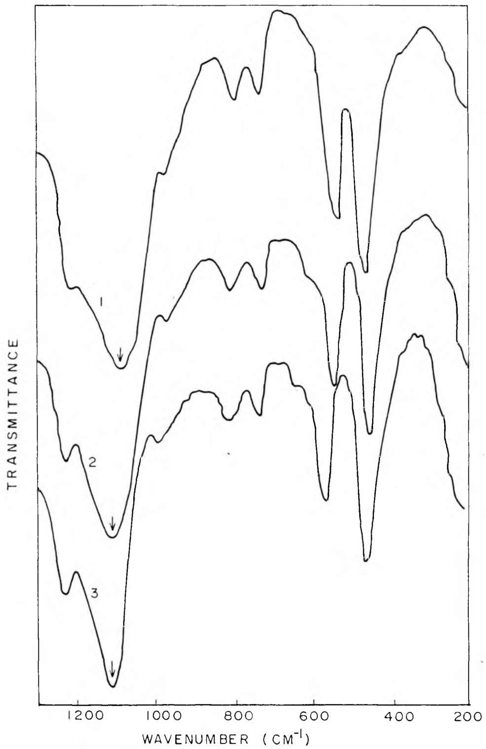
FIG. 2.17. INFRARED SPECTRA OF 1) Fe-EU-1 2) Fe 2 O 3 + SILICALITE 3) SILICALITE
