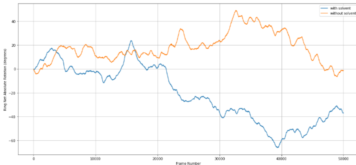
Figure 6.43. Plots showing net absolute rotation of the ring with and without solvent in the rotaxane system simulated at 1300 K in the presence of counterions.
