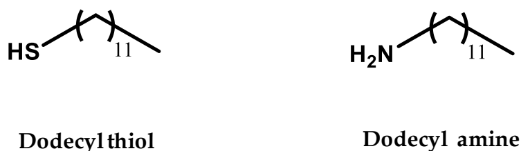
Figure 1.9: Thiol and amine was used as a DRA to demonstrate effect of metal-DRA binding strength during DR of Ag, Au and Pd NCs.
