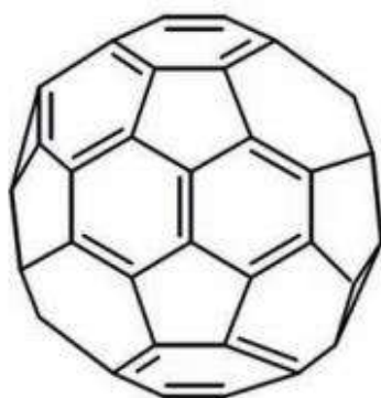
Figure 1.17. The pictorial representation of the buckminsterfullerene (Reprinted with permission, Copyright © 2012, John Wiley and Sons, License Number: 5314780410622).
