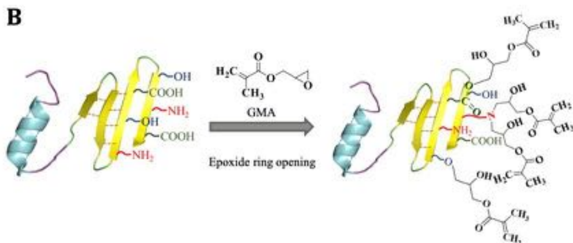
Figure 6-1 Schematic for the fabrication of SFMA A) fabrication of chemically modified SF with GMA; a. degumming of SF b. Washing of degummed SF fibers DI water; c. Dissolution of SF into 9.3M Lithium Bromide solution; d. Addition of GMA and TEA; e. Dialysis with Dialysis with DI water; f. lyophilization; g. lyophilized SFMA. B) Incorporation of functional methacrylate groups into SF by epoxide ring-opening polymerization reaction and a possible site for the modification includes -NH 2 , -OH and -COOH. 42
