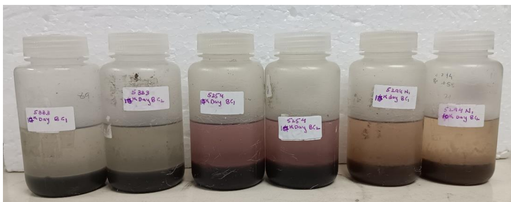
Fig. 27 Culture BCR10 in 5294, Extraction using ethyl acetate, carried out in duplicates, On the tenth day.
