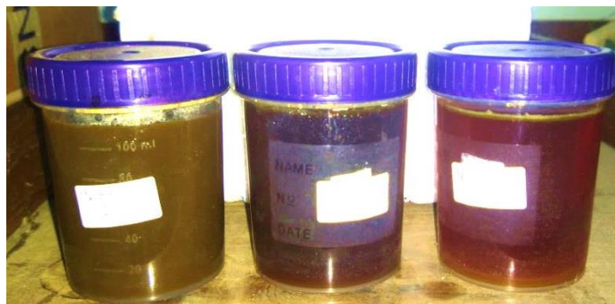
Figure 3.22 Reaction mixture of NAG hydrolysis in subcritical water at 250 °C at 5 MPa, 12.5 MPa and 25 MPa (from left to right)
