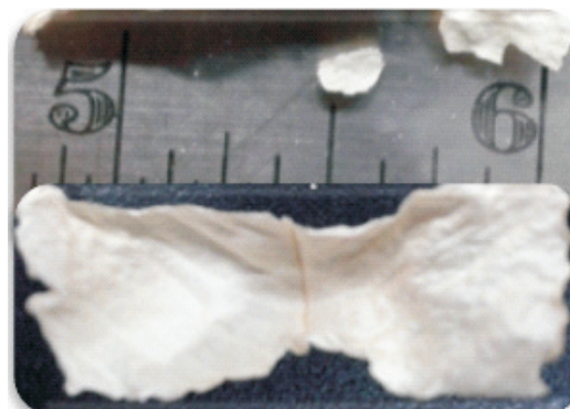
A typical cut-piece of fresh leaf from champa tree. Entire (above); a typical inorganic ZnO leaf (below)
