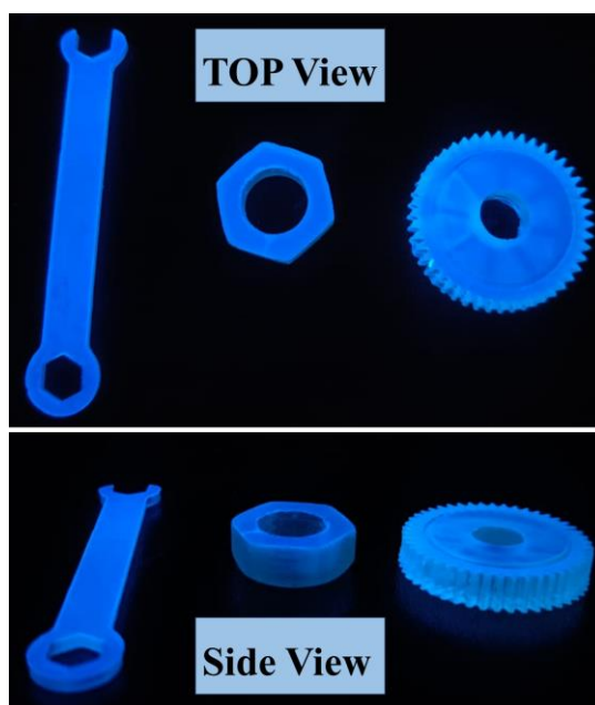
Figure 5.12 High-resolution 3D printed parts with BBOT dye
