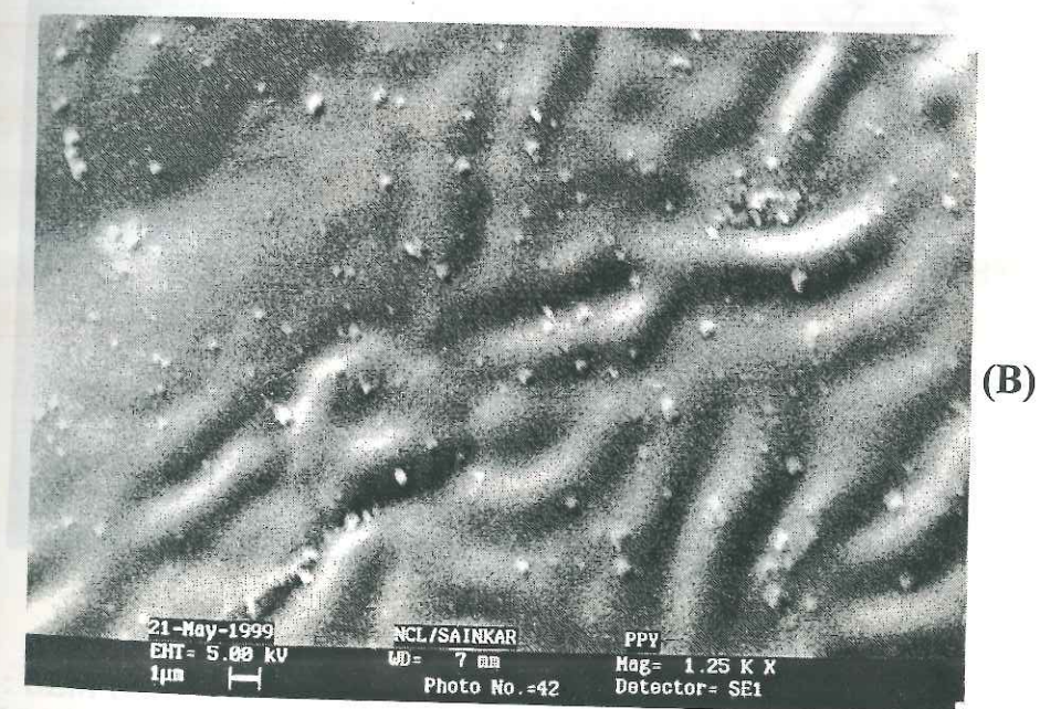
Figure (3.8) : SEM of the electrochemically as deposited Ppy film at 250x (A) and 1.25x (B) magnifications.
