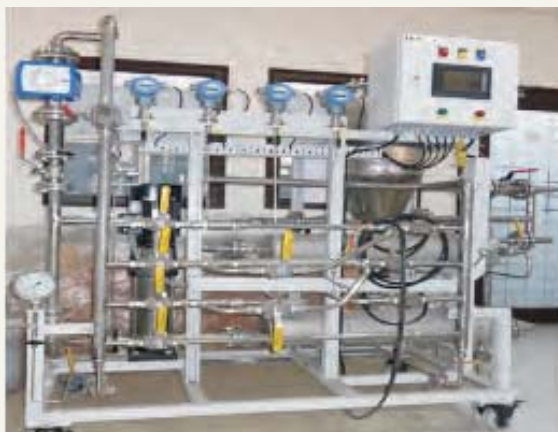
Cavitation pilot plant (Capacity: 1 m 3 /h)
