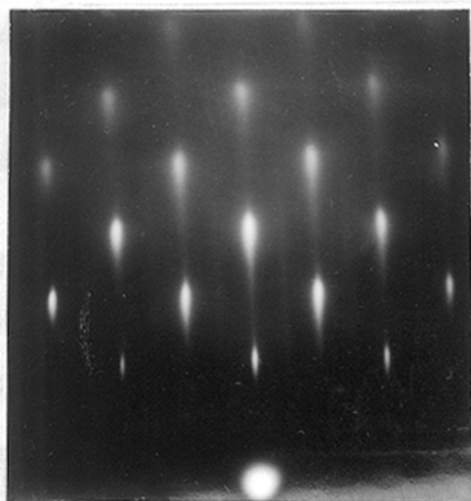
Fig.131 Silver electro- deposited from cyanide solution on copper (110) A/10, 5 sec. azimuth [001]_{Cu}
