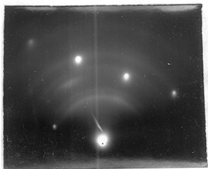
Fig.139 Platinum displaced on iron from M/2000 chloroplatinic acid
