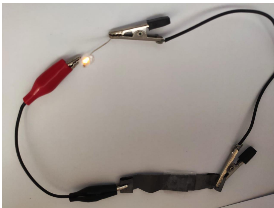
Figure 2.25. Quasi solid-state symmetric device demonstration after charging the device.
