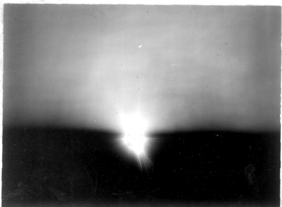
Fig 74. Electron diffraction pattern after mechanical polish- ing polycrystalline mild steel.
