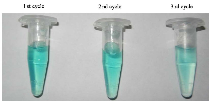
Fig. 2B.16. Images for TMB oxidation by fresh and recycled catalysts.
