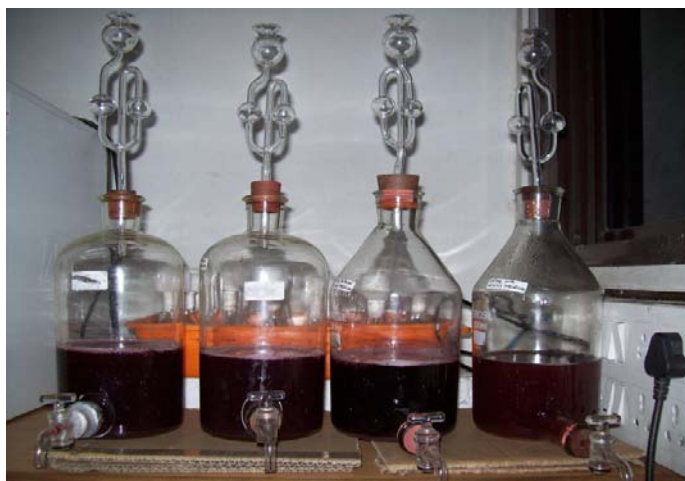
Figure 3.9 Laboratory fermentation of Shiraz variety Temperature; 15-20° C, Time; 15 d
