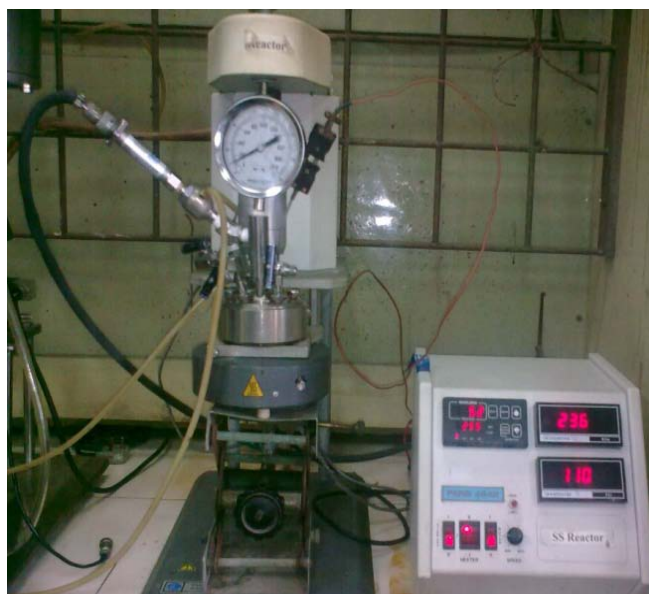
Figure 3A.2. Batch mode reactor used for depolymerization studies of lignin.
