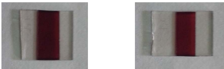
Figure 6. Dye loaded TiO 2 photoanodes
