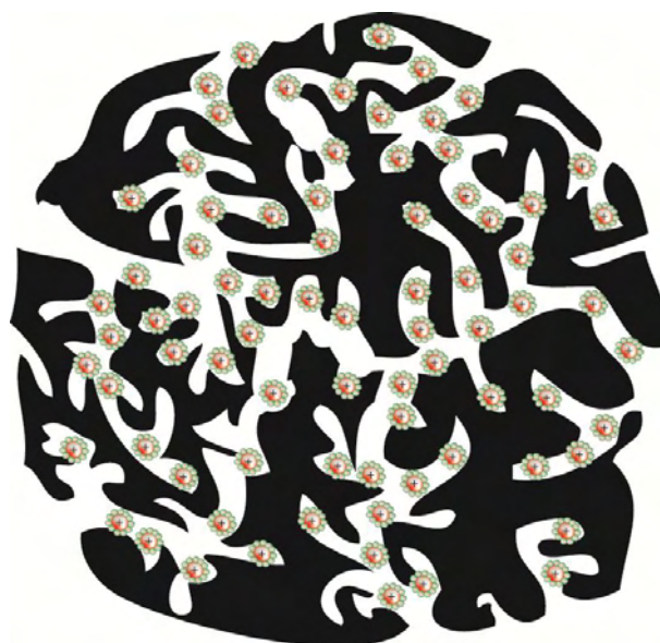
Figure 1.10: A schematic representation of the activated carbon sphere pore structure and possible EDL formed with the solvated cation.
