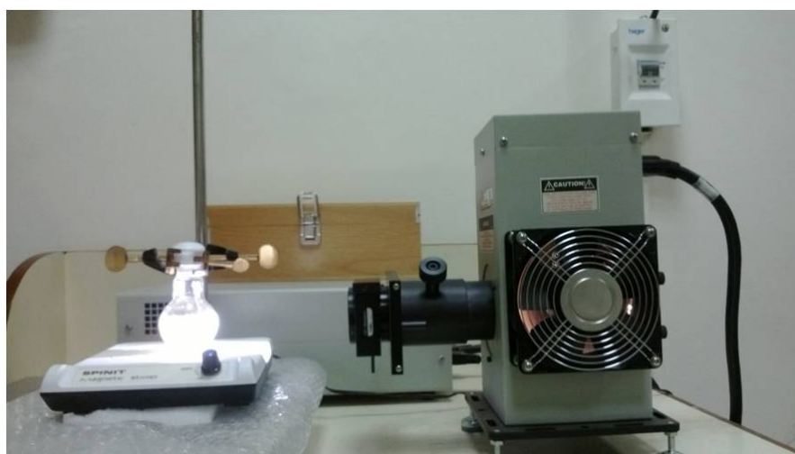
Figure 2.2. Photocatalytic reaction set up using solar simulator source
