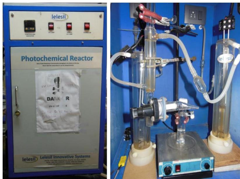
Figure 2.10. Reactor set up for photocatalytic water splitting which consists of a quartz cell having 70 ml capacity and it is gas closed by means of rubber septum. The light sources are inside the quartz jackets where cold water circulates continuously.
