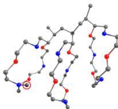
Figure 4.15 The optimized structure for the tri-aza pendant group case; there is one CH 2 pendant group in the alkyl backbone in the example shown above; the color scheme is the same as in Figures 4.5, 4.9 and 4.14.
