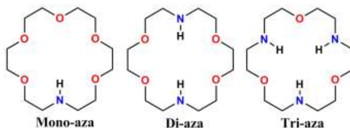
Figure 4.4 Chemical structures of the aza-18-crown-6 ether pendant groups that have been investigated in the current study.
